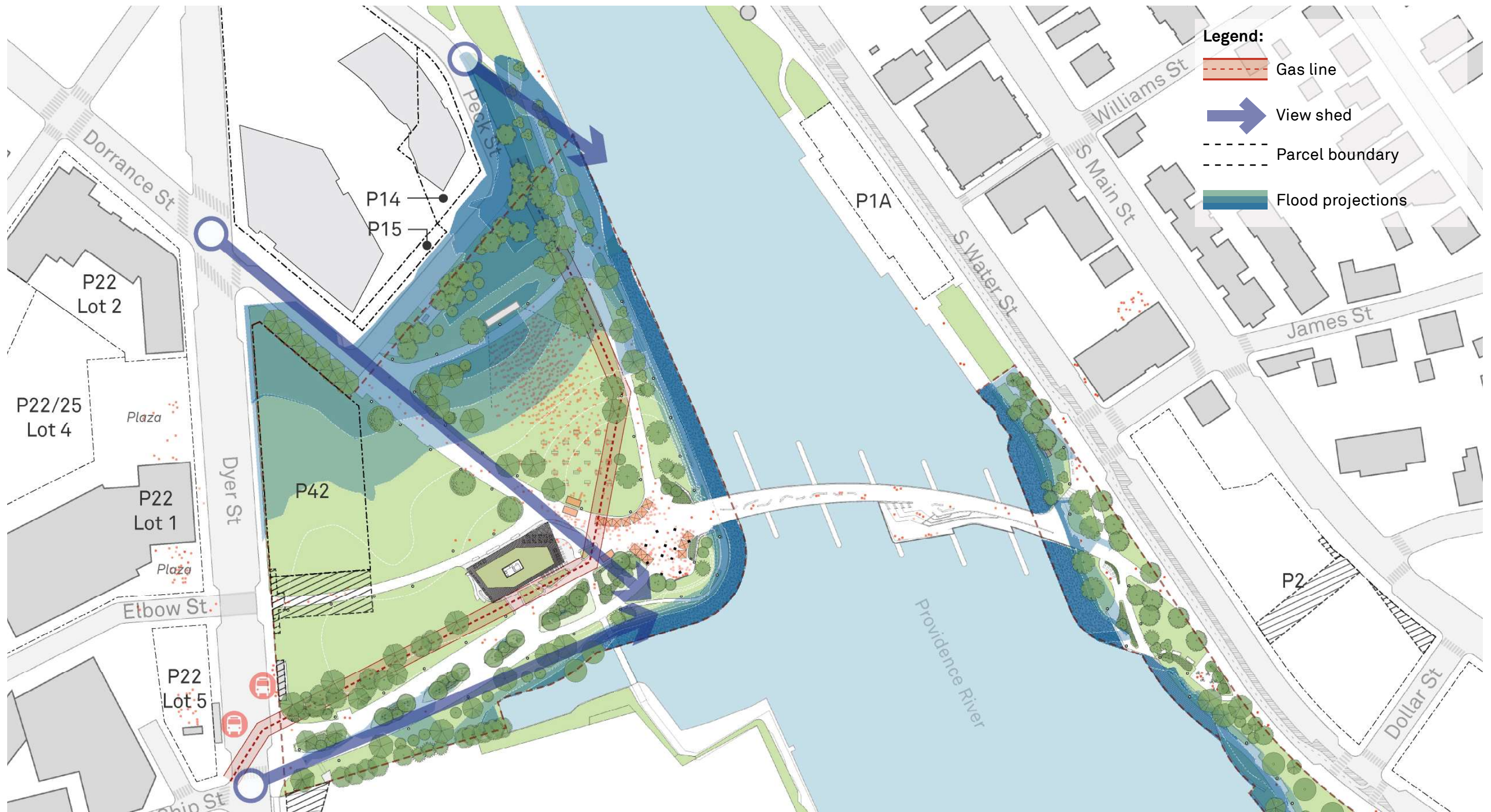
Site constraints include estimated future water levels, an existing high pressure gas line running beneath the site, and preserved view corridors that run through the park to the river.
